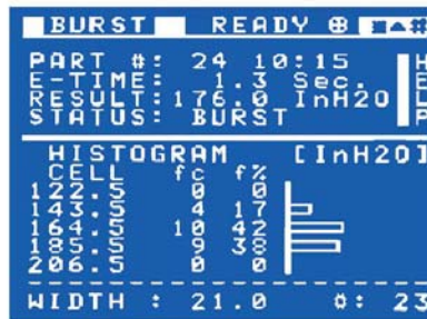
Accumulating test data are shown in histogram form to give a visual overview of your process.
