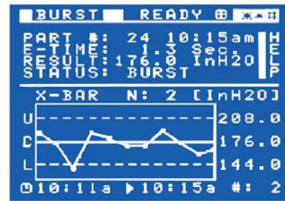
Ongoing test data are shown on a statistical control chart for tighter process control.
