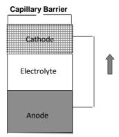
Oxygen enters the sensor through the capillary where it comes in contact with the cathode, and is immediately reduced to hydroxl ions:
