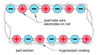
Finally Coulometric sensors, based on the electrolysis current of the water vapour absorbed in a hygroscopic material, are the technology of choice for various permeation instrument makers. Systech Illinois Instruments have been at the forefront in the development of these sensors for a number of years, which provide an economical yet potentially extremely sensitive solution.
