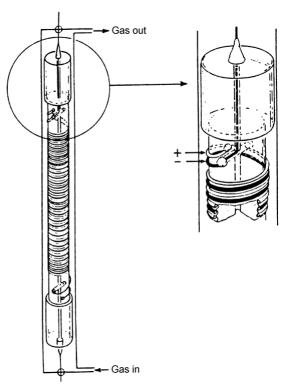
which is extremely hygroscopic. The moisture migrates through the film to the electrodes (platinum wires) where is it electrolysed. Oxygen is formed at the positive electrode and hydrogen at the negative electrode. The gases diffuse back into the gas stream where they are carried out of the cell. All of the moisture in the gas stream is consumed as it passes through the cell.
