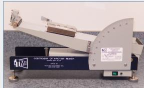
TMI offers two instruments and methods to measure static friction: The horizontal plane method and slide angle static friction method, shown above.
