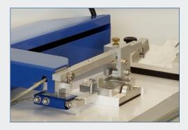
Testing Machines offers Model 32-25 Slide Angle and Model 32-76e Horizontal plane method for static and kinetic COF. Model 32-76 can be interfaced to GraphMaster PC software to record static/kinetic curve analysis and data storage.
