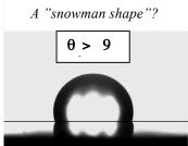
Converters, film extruders and printers need to measure quality and consistency of film treatment to insure proper liquid to substrate adhesion.
